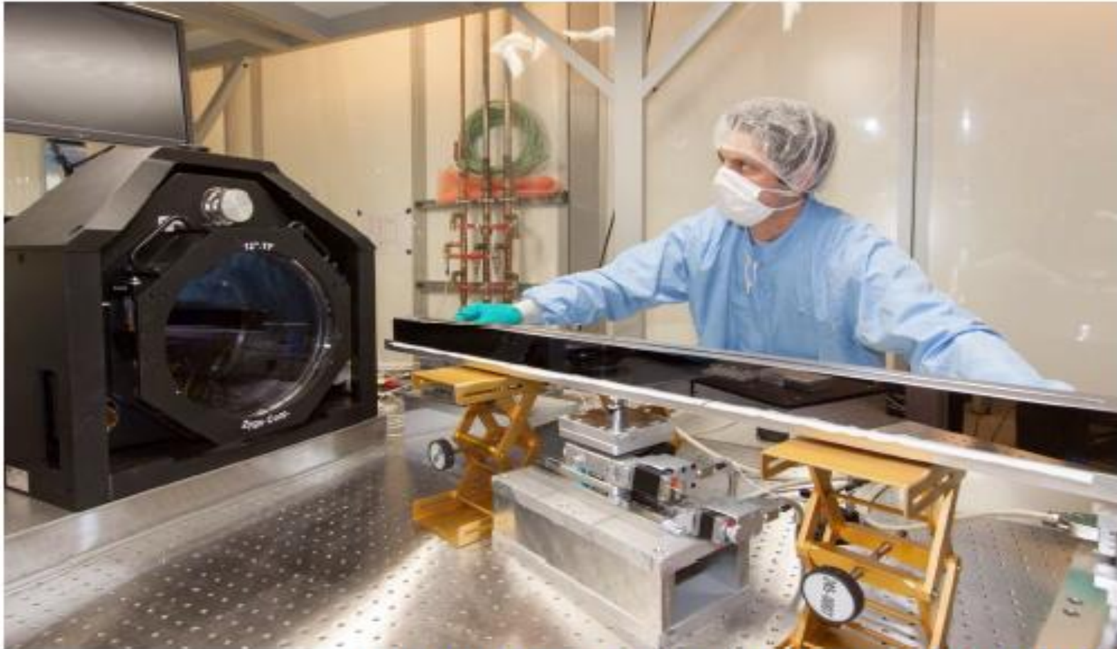
Metrology on first long JTEC mirror by Maurizio Vannoni
