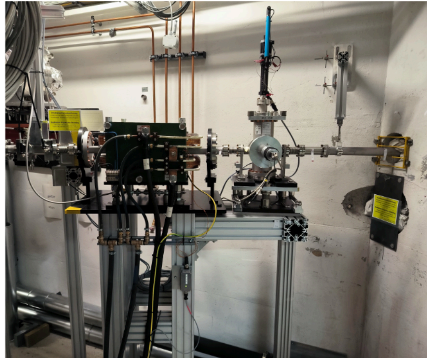
last bending dipole to parallelise to L-Weg
